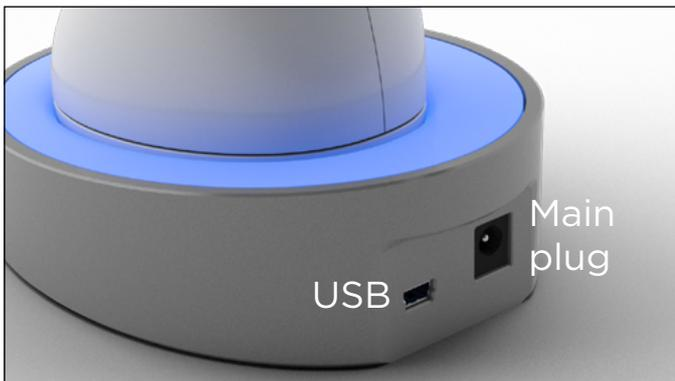
Before first use, the device must be charged. The charge can last up to 4 hours. For this, the device must be placed on its base and connected through the cable to a power outlet or USB.
