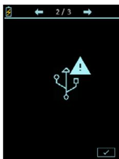
The USB connection failed. Check that the cable is well connected and then re-connect.
