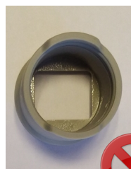
DAMAGED CALIBRATION TIP Internal and/or external shiny and sticky appearance
