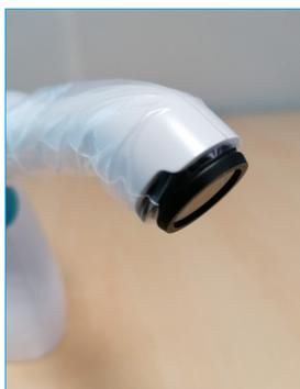
Before each utilization on a patient, place a protective sheath over the measuring head of the Rayplicker™.
