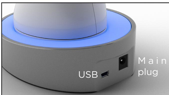
Before first use, the device must be charged. The charge can last up to four hours. For this, the device must be placed on its base and connected through the cable to a power outlet or USB.
