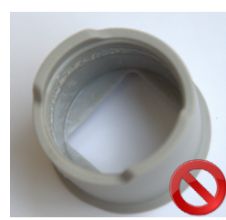
DAMAGED TIP Internal aspect and/or external shiny and sticky
