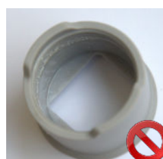
DAMAGED TIP Internal aspect and/or external shiny and sticky
